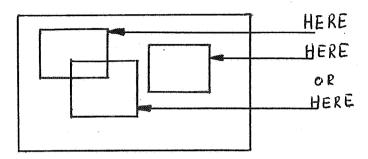
Thus with respect to controlling a plotter, the limits of the requested display space only defined the area to be used. Consequently, SET REQUESTED DISPLAY SPACE could equally well define the area in the lower left hand corner. Defining it aywhere else is just confusing.
